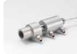
The air/water cooled housing allows the sensor to withstand ambient temperatures which exceed the normal 70°C limit. Air or water (depending on the degree of cooling required) flows into one of the fittings on the side and out of the other. To prevent condensation forming on the lens, the air/water cooled housing is supplied complete with an air purge collar. Please note, the air/water cooled housing must be ordered with the sensor and cannot be fitted by the user.
