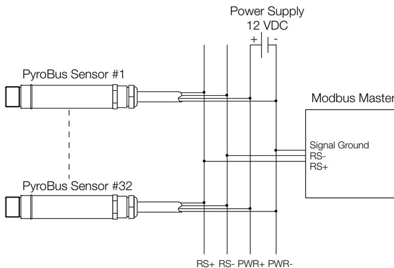
The PyroBus Series is a range of high quality, low cost, compact sensors which measure the temperature of inaccessible or moving objects and materials. They measure temperatures from -20°C to 500°C, accurately and consistently, with an outstanding response time of 240 ms.
