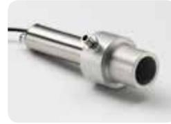
The air purge collar is used to keep dust, fumes, moisture and other contaminants away from the lens. Air flows into the fitting on the side and out of the aperture at the front.
