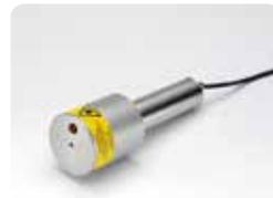
The Laser Sighting Tool screws onto the front of the sensor and indicates precisely where the sensor is aiming. Once the sensor has been aimed at the centre of the target and locked in position the Laser Sighting Tool can be removed. The laser is activated by means of a push button on the front of the tool which has a latching mechanism.
